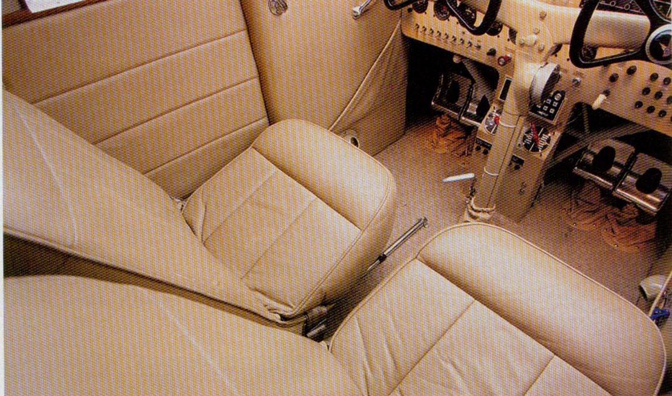
Inside this prize-winning Staggerwing is a leather interior with room for five. A modified fuel system places the selectors on the center pedestal.
